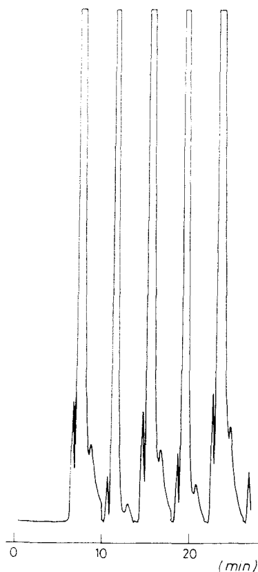
Figure 5. Preparative chromatogram of zopiclone showing several injections on a Kromasil C 18 100 Å (10 μm) column, 50 x 250 mm, in acetonitrile (100%) at a flow rate of 60 mL/min. Sample size: 300 mg. Pressure: 1.8 MPa.
